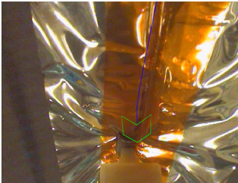
Fig. 10: Augmented reality display for satellite servicing, showing cutter goal position (green chevron) and virtual fixture path constraint (blue line)
